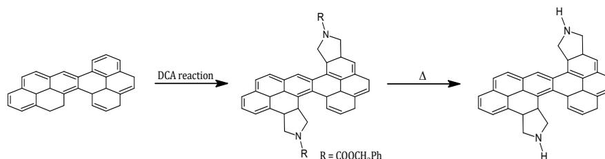
Figure 1: Schematic representation of the functionalization route of CNTs *via* 1.3 dipolar cycloaddition [4].
