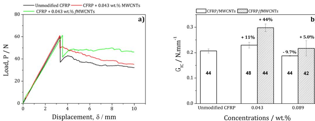
Figure 2: Representative load vs displacement curves a) and mode-I interlaminar fracture toughness ( $G_{IC}$ ) b), respectively.
