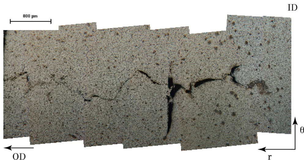
Figure 1: Characteristic crack path during SOHIC
