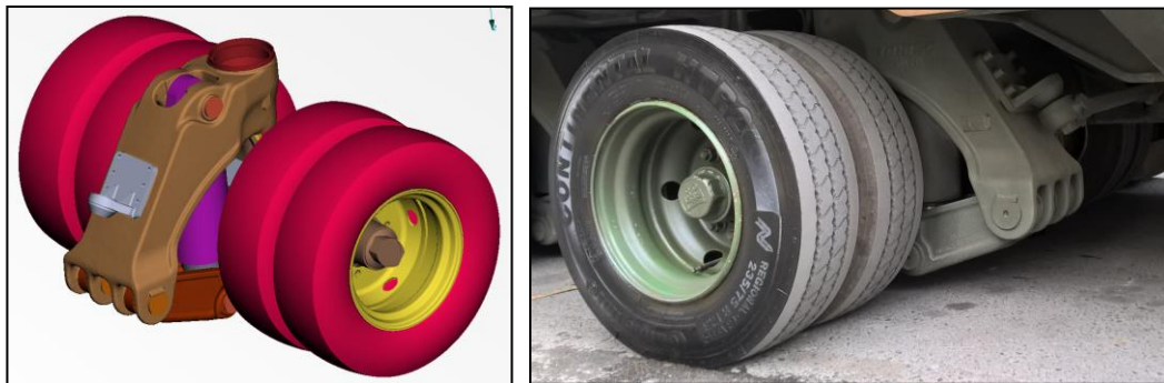
Figure 2: Finite Element Model of suspension system of a semi-trailer vehicle; real system.
