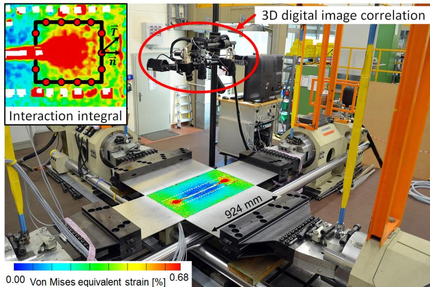
Figure 1: Biaxial testing of cruciform specimen supported by 3D digital image correlation
