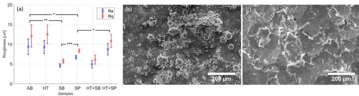
Figure 1: (a) Microscale surface roughness parameters; top surface SEM micrographs of (b) AB and (c) SP specimens (AB: as built, HT: heat treated, SB: sand blasted, SP: shot peened, HT+SB: heat treated and sand blasted, HT+SP: heat treated and shot peened)
